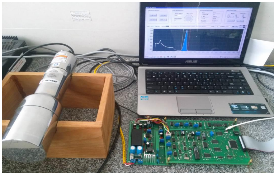
Fig.3. Diagram final assembly of multi-channel analyzer
