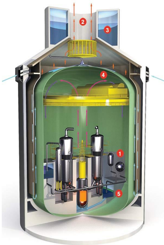
Fig.1. Performance of AP1000 Passive Containment Cooling System [2]
