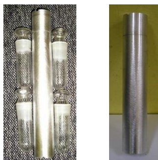
Fig. 3. Quartz ampoule and aluminum container for containing target.
