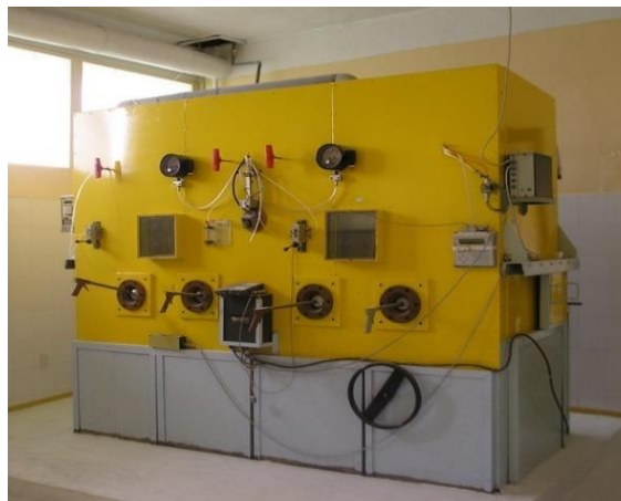
Fig. 7. ^{99\text{m}}\text{Tc} generator production line.
