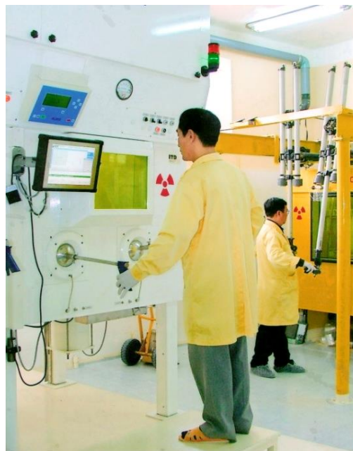
Fig. 6. ^{131}\text{I} isotope production line equipped in 2008 with 2 shielded cells.
