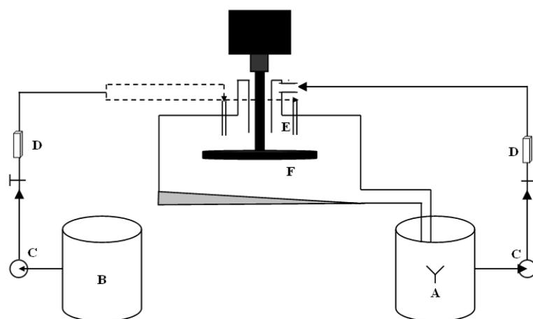
**Fig.1.** Experimental setup for preparation nano-silver using spinning disc reactor.
