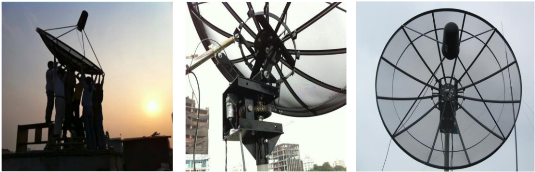
Fig.1. The VATLY radio telescope; left: installation; middle: close up view of the steering gear box; right: the dish and its sensor.
