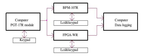
Fig. 3. Principle schema for measurement of the reactor power and period using PGT-17R module
