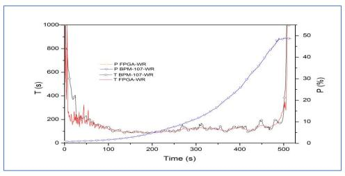
Fig. 6. Results of power and period measurements in the range from 0.5 to 50% Pnominal
