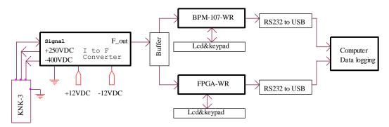
Fig. 5. Principle schema for testing the reactor power and period using KNK-3
