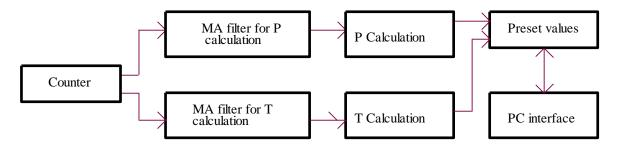
Fig. 2. Principle schema used for neutron flux measurement FPGA-WR
