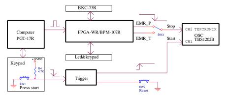
Fig. 8. Principle schema for testing response time of FPGA-WR and BPM-107R modules
