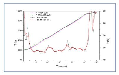
Fig. 7. Results of power and period measurements in the range from 50% to 80% P<sub>nominal</sub>
