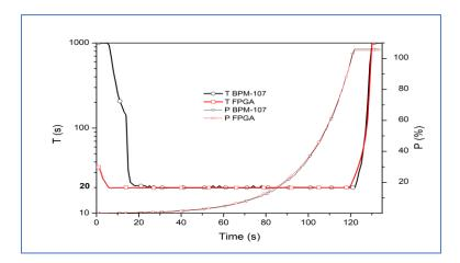
Fig. 4. Testing results of the BPM-107R and FPGA-WR modules using PGT-17R module with  $F_{WR}$  from 100 Hz to 50,000 Hz at the period of 20 s
