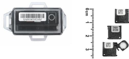
**Fig. 1.** OSLDs with InLight type (left side) and nanoDot one (right side)
