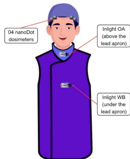
**Fig. 2.** The setting position of dosimeters
