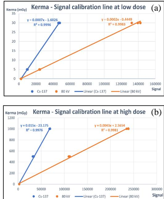
**Fig. 3.** Landauer calibration lines at low dose (a) and high dose (b)
