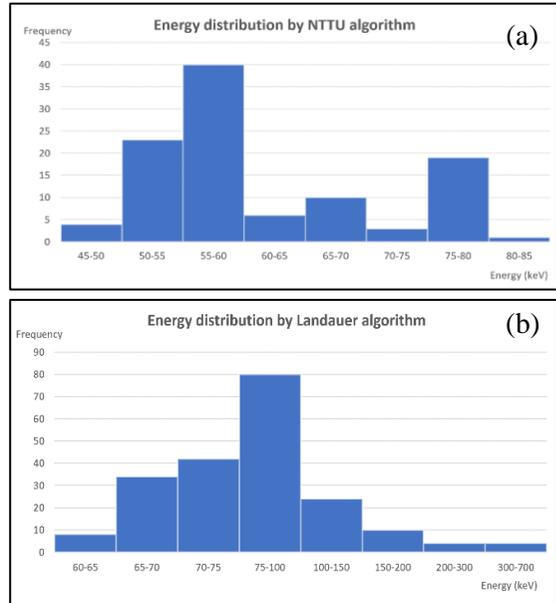
**Fig. 4.** Energy determined by NTTU (a) and Landauer (b) algorithms for OA dosimeter
