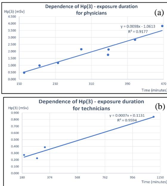
**Fig. 5.** Eye lens dose – exposure duration for the physicians (a) and technicians (b)
