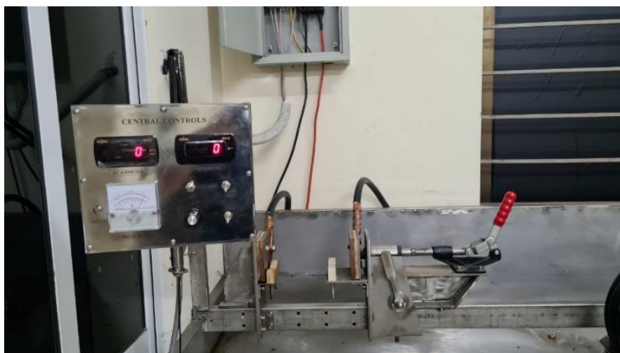
Fig. 14. Internal short circuit check
